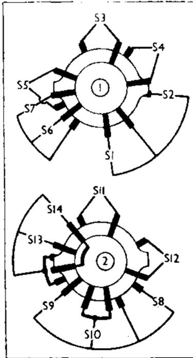
Switch diagrams, looking from the underside of the chassis, in the directions of the arrows in the under-chassis view.
