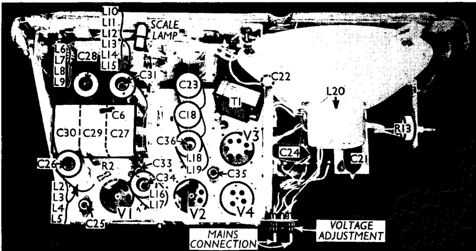
Plan view of the chassis. Each coil unit contains one trimmer, other associated trimmers being mounted on the chassis nearby. **R2** is inside the top cap connector of **V1**.
