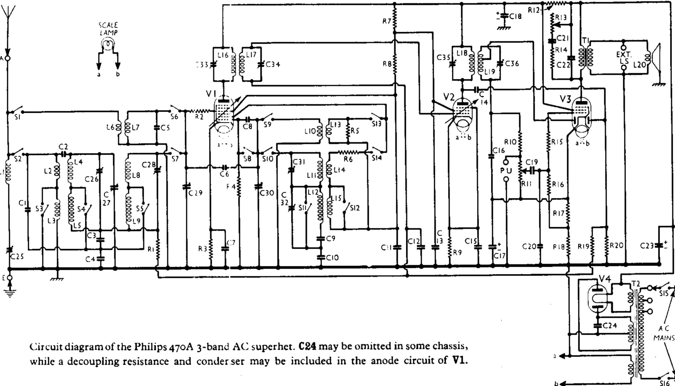
Circuit diagram of the Philips 470A 3-band AC superhet. **C24** may be omitted in some chassis, while a decoupling resistance and condenser may be included in the anode circuit of **V1**.
