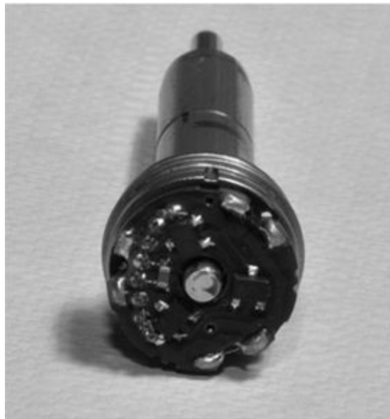
Figure 51: Hall sensors in a brushless motor
