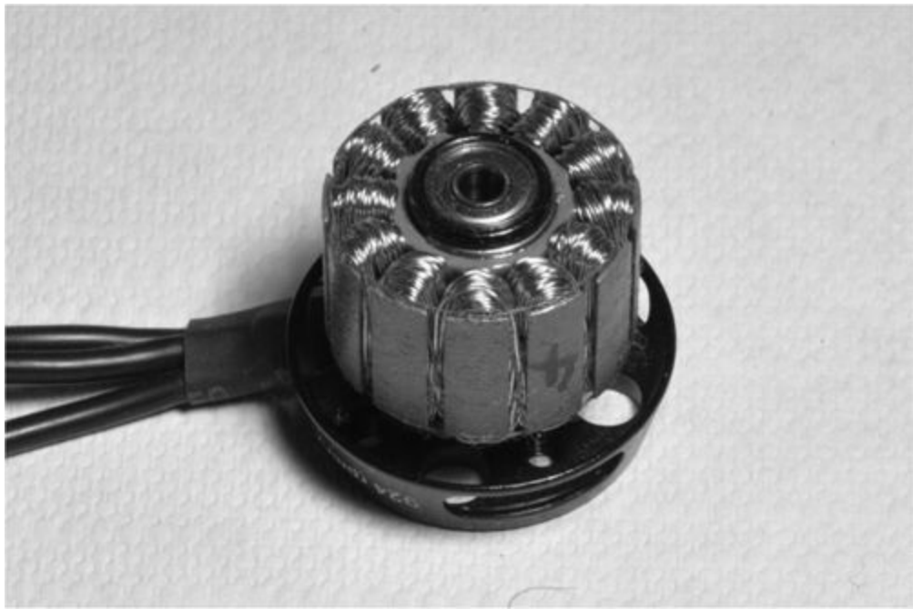
Figure 14: Stator of an outrunner
