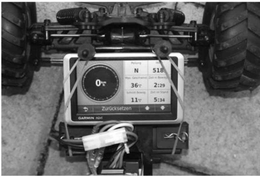
Figure 73: Speed measurement with GPS navigation device
