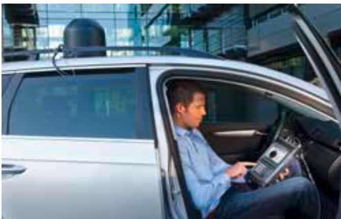
Commercial vehicle with installed R&S®MobileLocator ready for use. The operator controls the system via a laptop or tablet.
