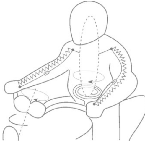
Figure 1.32 Rider impedance model.
